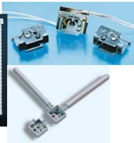
The zinc material aids the cord to pass smoothly through while a zinc pin locks the cord when activated. In this design the zinc die casting replaced a multi-piece steel assembly, reducing the cost and improving the operation. Many blinds also incorporate a die cast zinc gearbox to activate the tilting of the blinds.
